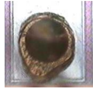
Aluminum splashing shorting to adjacent pad
