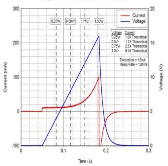
Ramp Test Data at -40°C, T545V107M016ATE016.
