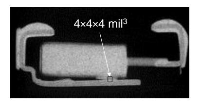
A part with significant crack at cathode attachment had ESR close to the average values.
