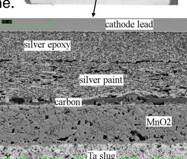
Degradation of ESR is typically attributed to delaminations and increased resistances at interfaces in cathode layers.
