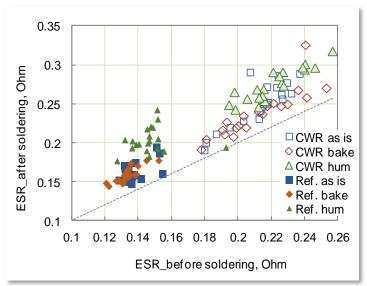
Two types of CWR29 capacitors (CWR and ref.) were reflow soldered after different preconditioning: (1) "as is" after long-term storage at room conditions, (2) after bake at 125 ° C for 15 hr, and (3) after 85 °C, 85% RH for 100 hr.
