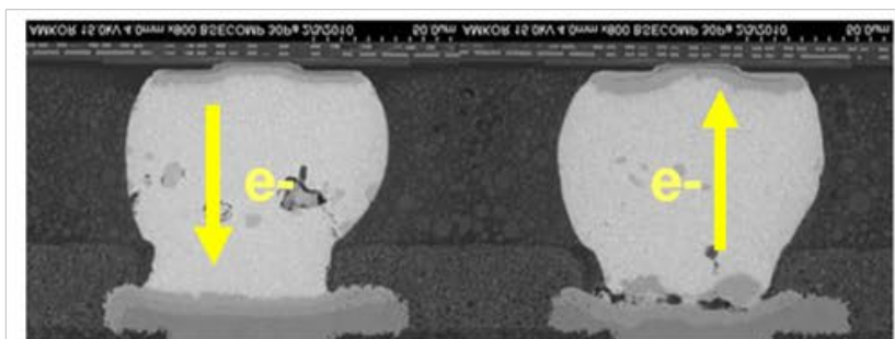
Figure 9: Failure mode for High Pb bump showing failure on substrate (cathode) side
