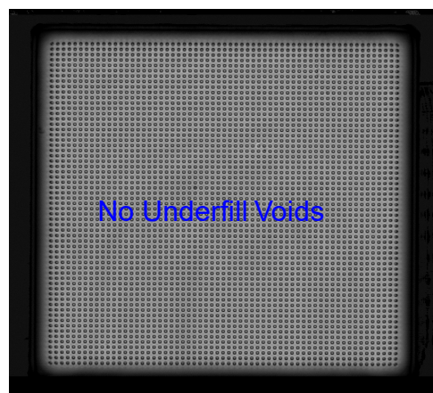
Vacuum Pressure Curing
