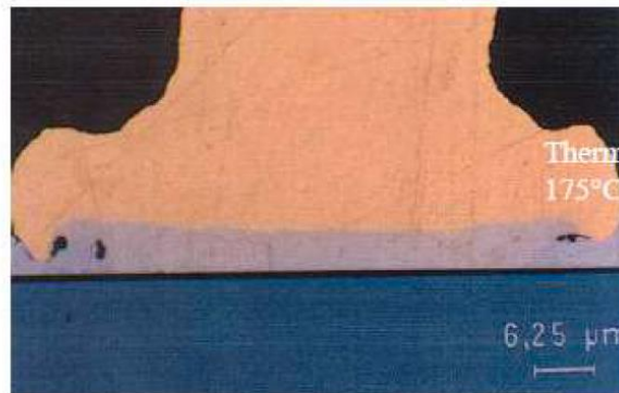
Intermetallic Penetration - AlSi-Au Bond (aged 200 hours at 200°C)
