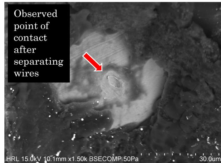
Laser ablation was successful in sufficiently uncovering the area of interest, revealing the failure site (upper left). The wires were separated, and subsequent inspection identified a breakdown of the wire insulation due to abrasion (upper right).
