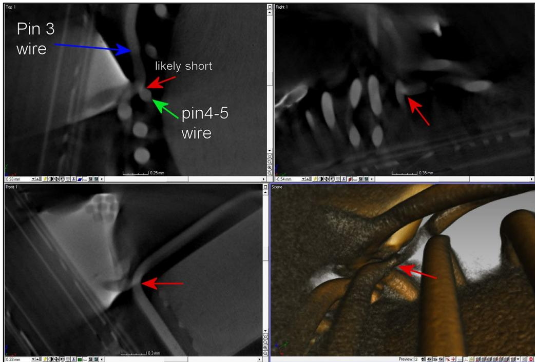
Detailed CT examination of the area indicated by IR hot spot detection revealed a single location where two wires from opposing windings made possible contact, tucked behind the solder joint on the substrate.
