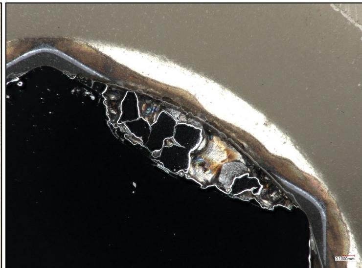
The location of this damage is consistent with failure due to a reverse biased over-voltage event, but the failure history is important in this case.
