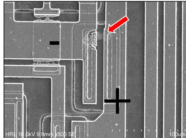
In the image to the right, the extent of damage was too severe to determine the true cause of failure. The root cause could only be speculated based on the severity of the damage in the output transistor.
