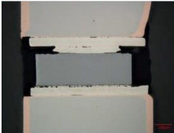
Optical image of cross section: glass body diode Image Source: Integra Tech
