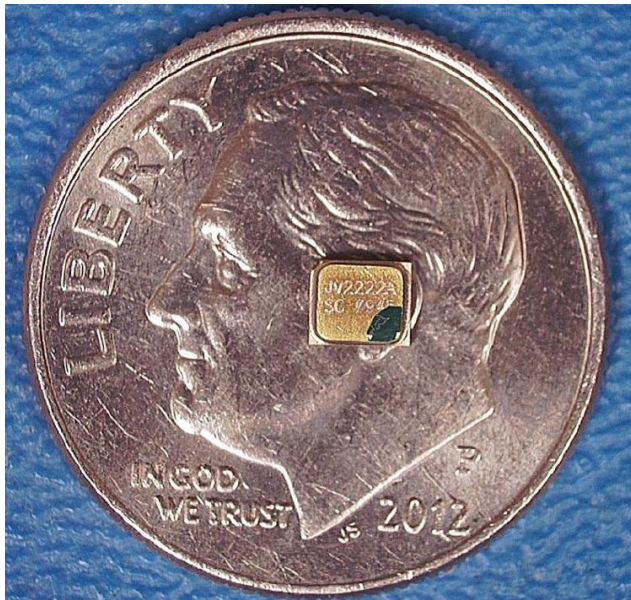
Transistor UB package failed due to moisture and corrosive material ingress through a hole in the lid Image Source: NASA GSFC
