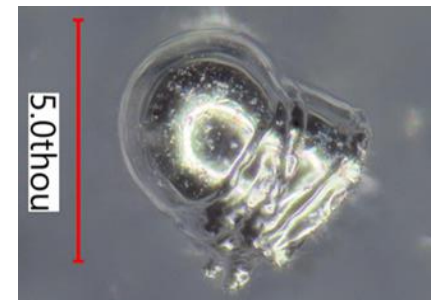
Examples of particle captured after PIND failure Image Source: NASA GSFC
