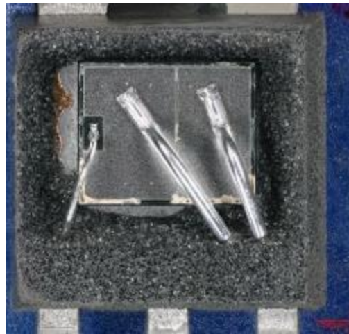
Decapsulated plastic encapsulated device with aluminum (Al) wirebonds Image Source: Integra Tech
