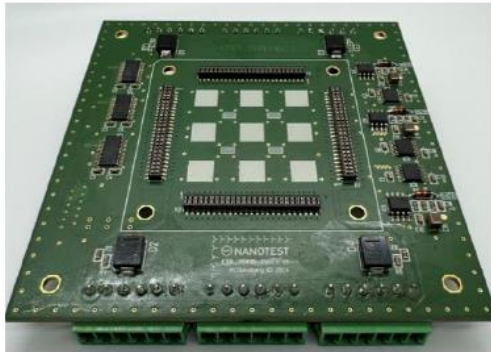
Electronic test board for TTV (adapter board with sense current and MUX)
