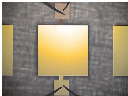
1000x1000 \mu\text{m} C = 1.6 \text{ nF}
