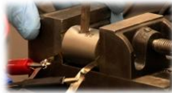
Puncture while charged and cycling
