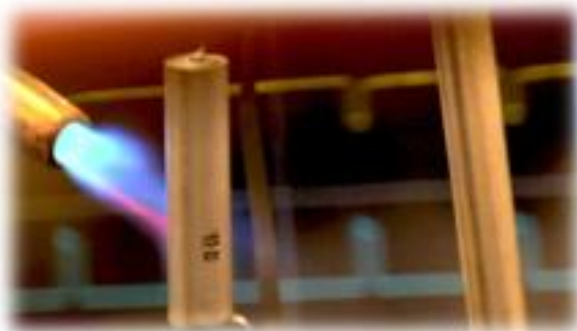
Blow Torch Test while charged and cycling
