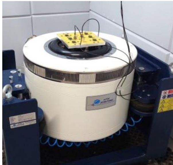
Pic. 10 Z-Axis Vibration Test
