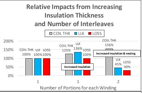
Increasing insulation thickness between windings is not volume efficient means to enhance leakage flux when increased nesting is required for reduced coil loss.
