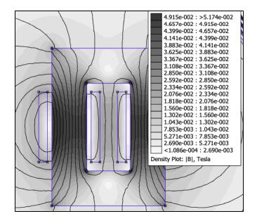
Add laminated core to enhance leakage flux with improved control.
