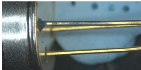
Fig. 4 Transistor produced in 1991, with corrosion on th lead and the body.
