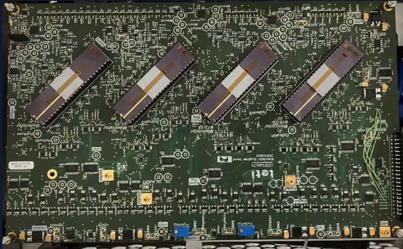
AI circuit board equipped with four spin-memristor ceramic packages
